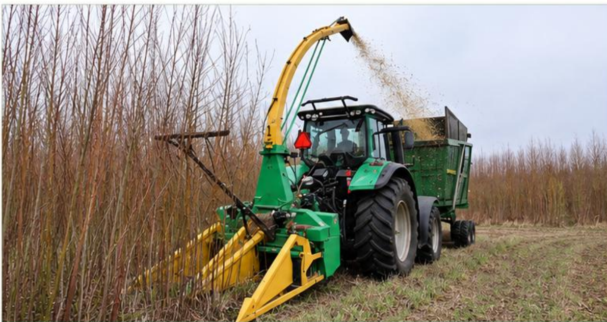
Mechanised cut-and-chip harvesting of short-rotation coppice willow
