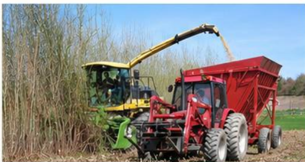
Cut-and-chip harvesting with forage harvester and trailer
