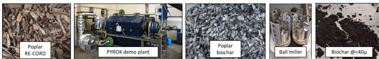
Figure 15: Schematic representation of the production chain of biochar with a particle size <40 μm.
