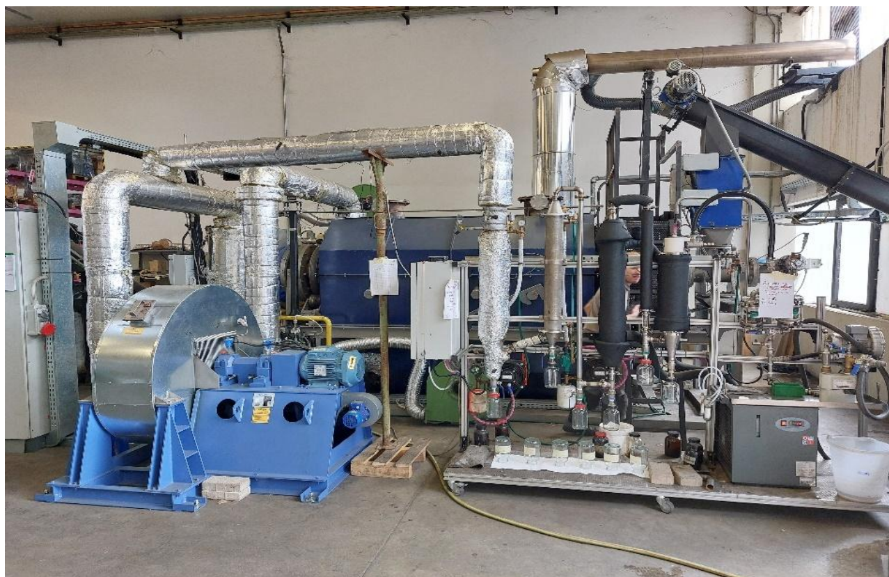
Figure 11: "PYROK" pyrolysis unit with vapor condensation system for sampling.
