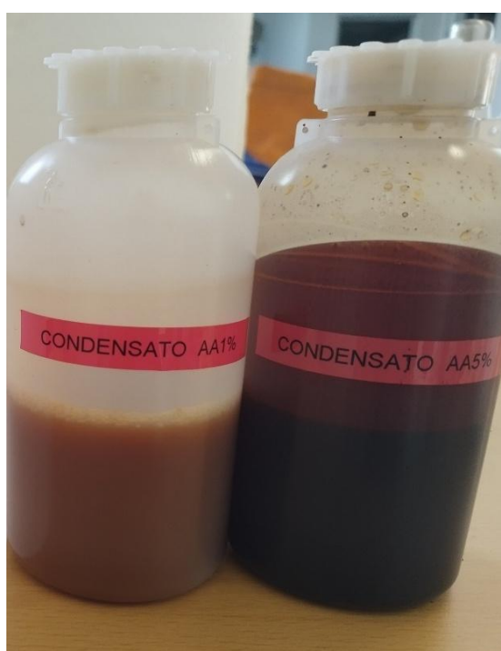
Figure 29: condensates appearance after dilution to specific acetic acid content (1%wt on the left and 5%wt on the right).
