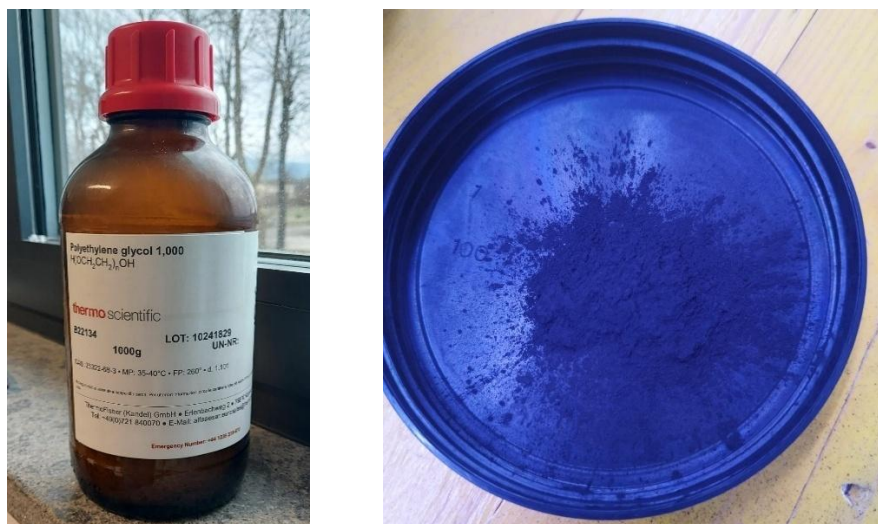
Figure 18: Polyethylene glycol (PEG) used as binder material (left) and milled biochar (right), used for seed coating.
