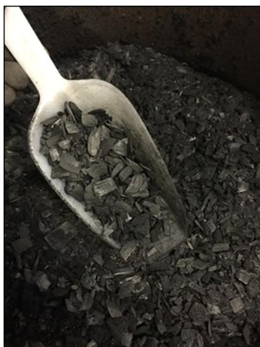
Figure 13: Poplar biochar produced in RE-CORD demo-plant
